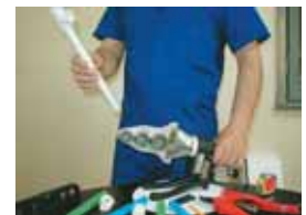
4; Join pipe and fittings. Finished! 100% safe welding
